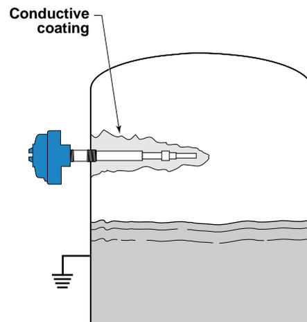
The probe's ACTIVE and GUARD sections operate at the same potential, thereby eliminating the path from the active section to ground at the tank wall. The unit therefore shows no alarm condition.
