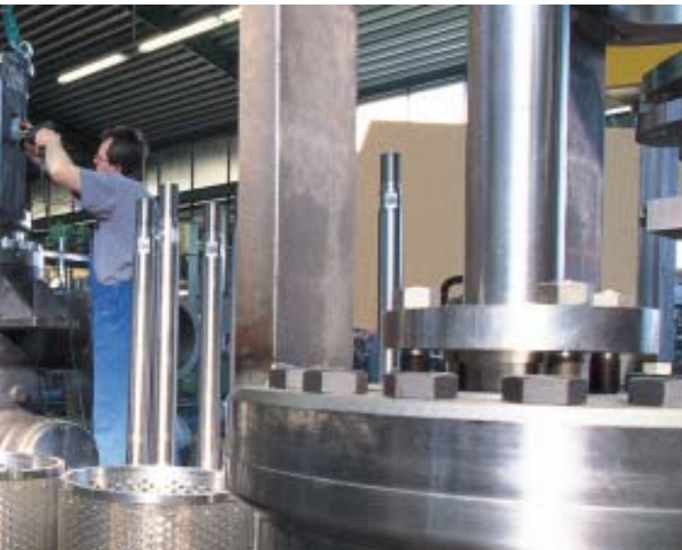
Assembling and checking the industrial valves, which may weigh over a ton, requires great precision and fine working.
