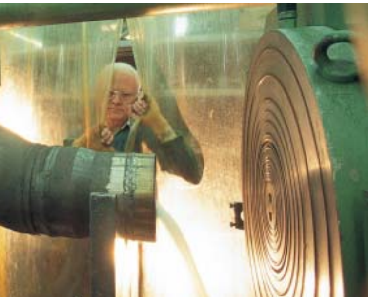
All HORA-valves are subjected to a pressure test of their seat and body tightness.
